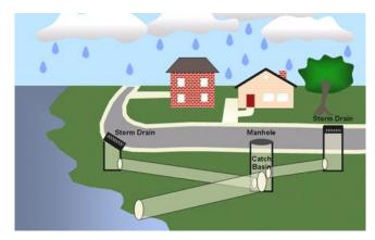
The storm drain system is a series of inlets, pipes, gutters, and ditches which carries <u>untreated</u> rain water away from streets and other paved areas and into nearby waterways.
